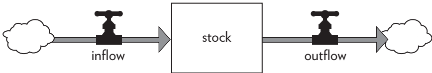
Figure 1. How to read stock-and-flow diagrams. In this book, stocks are shown as boxes, and flows as arrow-headed “pipes” leading into or out of the stocks. The small T on each flow signifies a “faucet;” it can be turned higher or lower, on or off. The “clouds” stand for wherever the flows come from and go to—the sources and sinks that are being ignored for the purposes of the present discussion.
